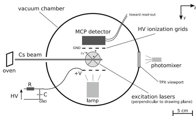
**Fig. 2** Illustration of the experimental caesium beam setup.
