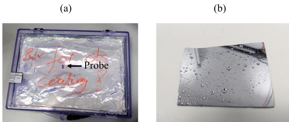
Figure 34: (a) Picture of a colloidal probe in a casing. The interior of the casing is covered with aluminum to prevent the OTS' reacting with the plastic walling. (b) Picture of water droplets deposited on an OTS' coated wafer.
