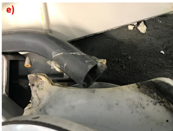
Appendix A1: Damaged LaboPol-5 polishing machine before repairs (a), with close-up images showing the casing (b), polishing wheel and bowl (c), chemical damage to the interior and screwhead destruction (d) and loss of seal between bowl and waste pipe (e).
