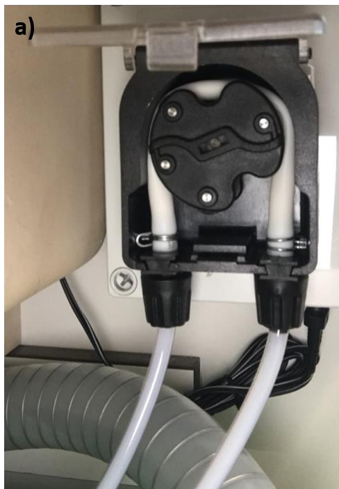
Appendix A3: Peristaltic pump (Verderflex Peristaltic Electric Operated Positive Displacement Pump 0.24 L/min, 12 V) to produce flow of polishing slurry (a) and a SUBA X Perf II 08 polyurethane-impregnated polyester polishing pad (b) for use in combination with a LaboPol-5 polishing machine for chemical mechanical polishing.
