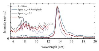
Figure 3.5: Spectrum produced with 2-µm laser light (red line) compared to the radiationtransported reference spectrum for a peak optical depth value of  $\tau_p = 2.2$  (gray line, barely distinguishable from the red line). Reference and 2-µm-driven spectra were both obtained using a droplet diameter of 30 µm. Also shown is a spectrum obtained using a 10-µm CO<sub>2</sub> laser that represents the case of small optical depth (reproduced from Ref. [111]).
