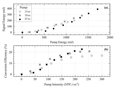
Figure 1.5: (a) MOPA output, plotted as pulse energies at the signal wavelength of 2090 nm, as obtained by varying pump energies at three different pump pulse durations. (b) Conversion efficiencies for different pump intensities, again for the three different pump pulse durations. The conversion efficiency is defined as signal energy divided by pump energy. Error bars are smaller than the markers.
