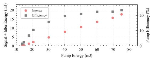
Figure 1.2: Combined signal and idler energies from the OPO as a function of the input pump energy (for a box-shaped pump pulse of duration  $\tau_p = 27 \text{ ns}$ ). The corresponding efficiency for conversion summed over both signal and idler is also indicated. Error bars are smaller than the markers.
