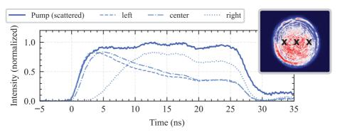
Figure 1.8: Temporal profile of the pump pulse resolved across the spatial beam profile. The blue solid line shows the temporal trace of the scattered light, i.e. representative of the full beam. The dashed/dotted lines show traces recorded with a 200 µm pinhole mounted in front of a photodiode to obtain spatially resolved traces at left, center, and right locations as indicated in the inset figure.
