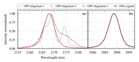
Figure 1.10: (a) Spectral analysis of the OPO idler output wave for three different cavity alignment conditions. (b) Spectrum of the signal beam of the OPO alignment 3 in (a) after amplification in the MOPA stage.
