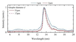
Figure 3.4: Spectral emission from tin plasmas produced with 1- and 2-µm laser wavelength for small and large droplet diameters at laser intensities of 2.4 and  $1.1 \times 10^{11}$  W/cm<sup>2</sup>, respectively.
