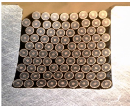
Fig. 152 Cut through of undulator winding, showing the winding stack
