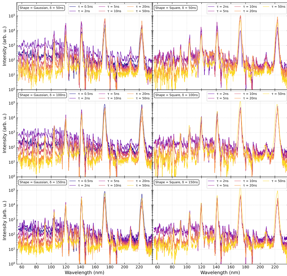
Figure 4.8: HHG spectra for complete parameter space comparing pump pulse lengths \tau . Pump pulse envelope shape and delays \delta are indicated for each subplot.
