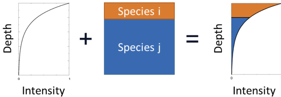
Figure 2-6 Schematic representation of the XPS overlayer determination: The left panel shows the decay of the measured intensity as a function of depth, the middle panel illustrates an overlayer of i on a bulk of j, and on the right their combination shows the signal arising from the overlayer in orange and the substrate in blue
