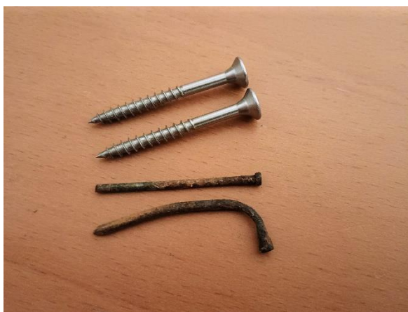
Figure 1-5 New metal screws, and old oxidized metal nails.
