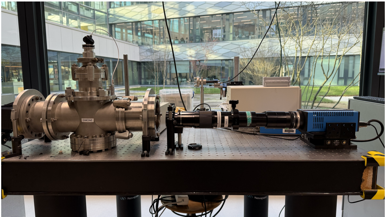
Figure 5.11: A new setup is developed/implemented to operate the microdroplet generator in a non-atmospheric environment. The camera (PCO-4000) is equipped with a long distance microscope (K2 DistaMax), with a working distance of 228 – 388 mm. First tests have shown that a pressure of 20 mbar can be achieved.
