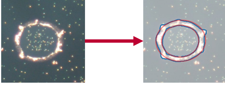
Figure 6.2: A 10 nm thick gold layer on borosilicate glass illuminated above the ablation threshold. The delaminated ablation edge creates an inner and outer contour as is shown on the right side.
