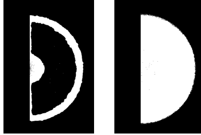
Figure 2.7: Thresholded image for an FF=0 and FF=1 structure. These images are used to determine the area of the void, which is required to normalize to when determining the FF of structured voids.
